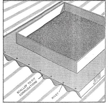
Rooflight unit can now be rivetted or screwed to upstand, with a gap of no less than 10mm above base of upstand.
