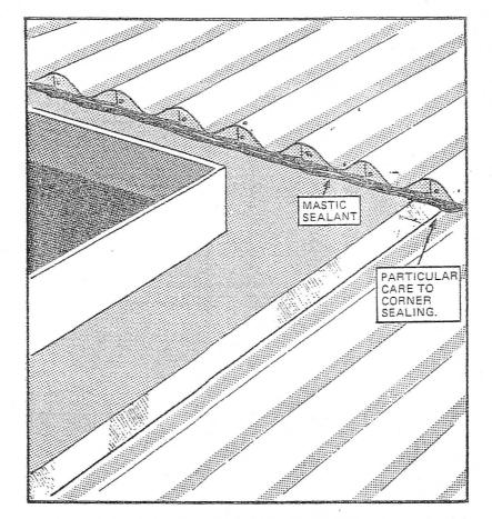
Lower edge of upstand flashing, should be either scalloped to suit corrugations, or carefully beaten to mould to sheet profile.
