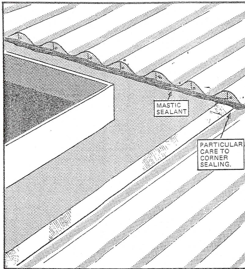
**7** Lower edge of upstand flashing, should be either scalloped to suit corrugations, or carefully beaten to mould to sheet profile.
