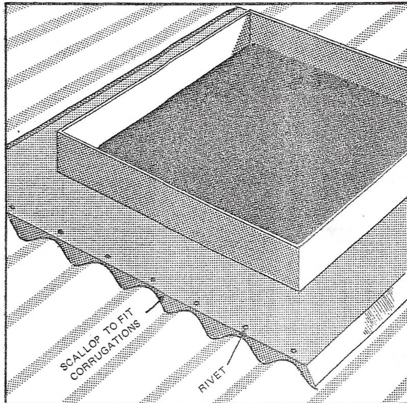
**8** Rooflight unit can now be rivetted or screwed to upstand, with a gap of no less than 10mm above base of upstand.
