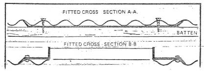
Turn up top-edge of upstand tray, and slide under roof sheeting and over batten at top edge of opening. Lay down over opening.
